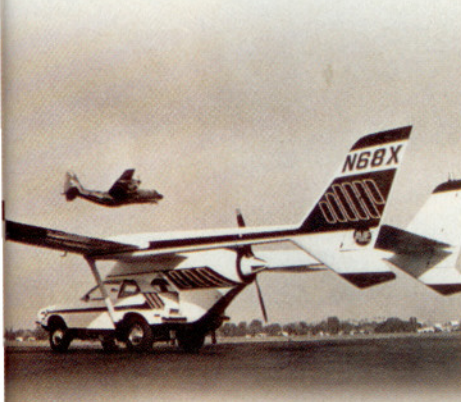
Molt Taylor with his first "Aerocar," built in 1949 (far left). The "Mizar" was developed by Henry Smolinski at Advanced Vehicle Engineers of Van Nuys, California. Its design was a Ford Pinto mated to the airframe of a Cessna Skymaster.
